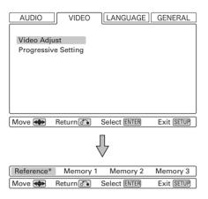
Near the bottom of the display, a row of four options appears: Reference, and three memory settings (Reference contains the factory default settings and the three memories can be used to make video settings for different monitors, types of program material, etc.).
